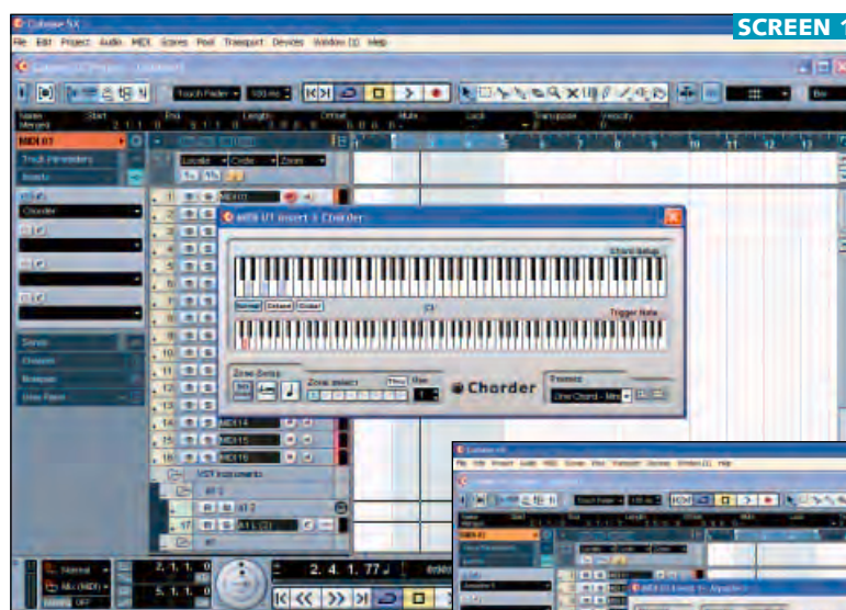
SCREEN 1 The Chorder allows you to assign a whole chord to individual keys
